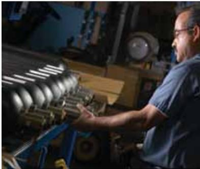
Every accumulator is pressure tested before it ships to the customer.
